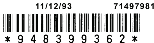
3 OF 9 BAR CODE SYMBOLOGY SIZE REQUIREMENTS FOR HIGH DENSITY BAR CODE 9.4 CHARACTERS PER INCH (CPI) (SCALE ENLARGED FOR CLARITY)
